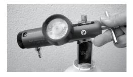
> Tighten the hand-screw clockwise to hold the regulator on the neck of the cylinder. Never use excessive force or tools to screw the regulator on to the cylinder
