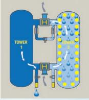
Dessicant dryers are commonly used to remove moisture in Medical Air production. All makes and models employ activated alumina and/or molecular sieve, both of which attract moisture and carbon dioxide.
